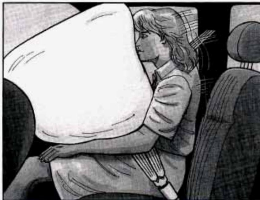
The driver's side impact air bag is in the driver's door.
