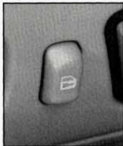
Press the power door lock to lock or unlock all the doors at once. The rear power door locks provide a lock only function as a convenience feature. For safety reasons, they will not unlock the doors.
