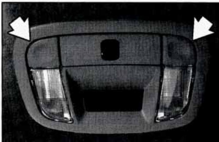
These lamps are located in the front overhead panel. Press the button to turn them on. Press it again to turn them off.
