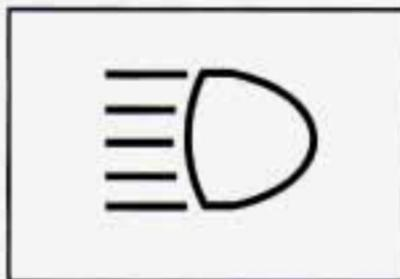
Pull the turn signal lever all the way toward you and then release it to change the headlamps from low beam to high or from high beam to low.
