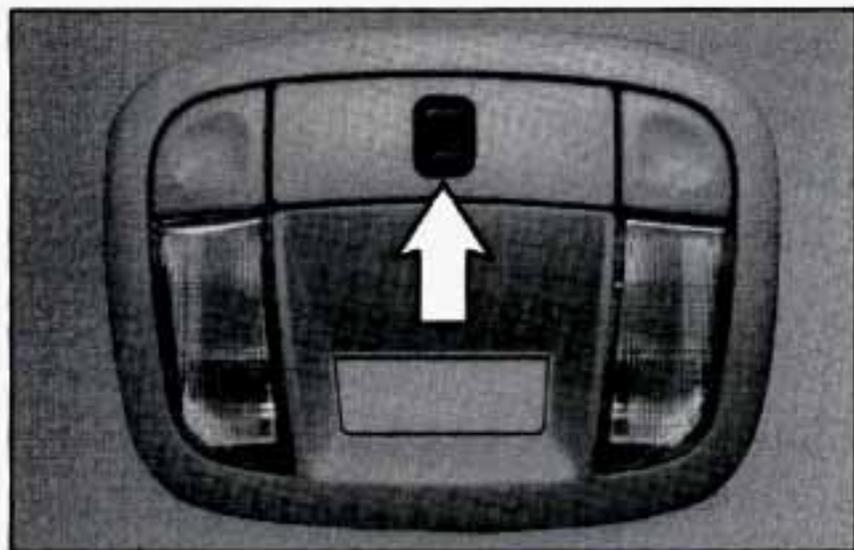
The control switch only works when the ignition is on or when the Retained Accessory Power (RAP) is active.
