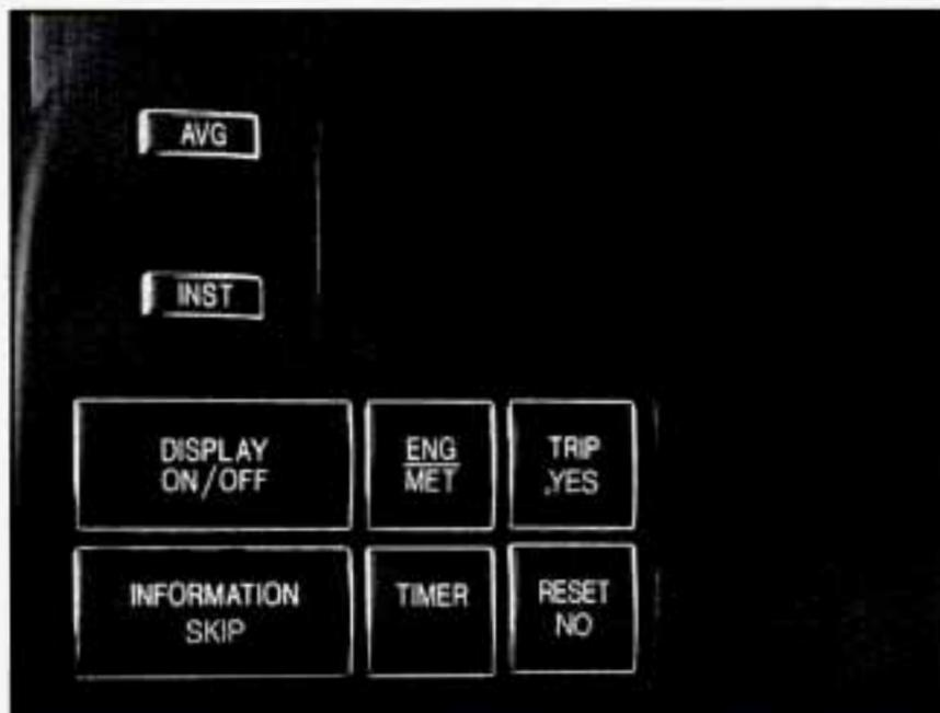
**DISPLAY ON/OFF:** Pressing this button will turn off the Driver Information Center (DIC), Electronic Climate Control (ECC), fuel data center, the fuel gage, trip odometer and odometer. While the displays are off, pressing the INFORMATION button will only turn on the DIC. If the TRIP button is pressed or the fuel level falls below 4 gallons (15.2 L), all of the displays will come back on.
