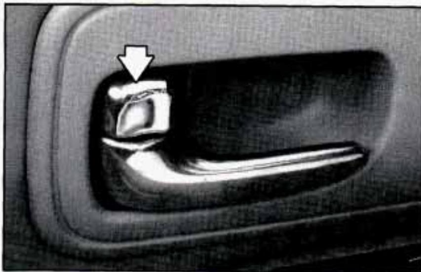
Rotate the manual lock lever forward to lock the door from the inside. To unlock the door, rotate the lever rearward.
