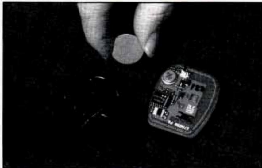
3. Remove and replace the battery. Insert the new battery as the instructions under the cover indicate.
