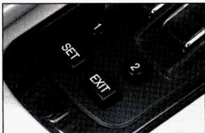
Automatic seat and mirror movement will occur if the Remote Keyless Entry (RKE) transmitter is used to enter the vehicle. The number on the back of the transmitter corresponds to the 1 or 2 seat and mirror position.
