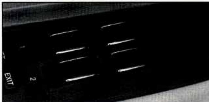
The controls are located near each window. Press the control forward to raise the window and press rearward to lower. Note that the second rearward position on the driver's control operates the express-down window feature.
