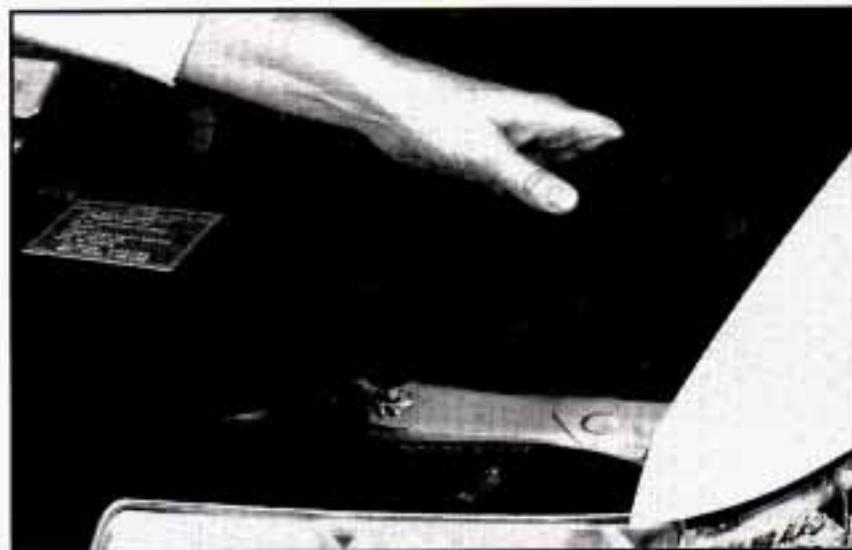
1. To access the headlamps, lift the cover as shown.
