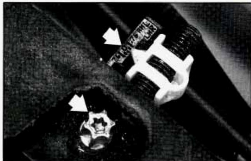
2. Check the vertical headlamp aim first. Keep in mind that your vehicle needs to be on a level surface. Turn the vertical aiming screw until the bubble inside the level is centered at "0."
