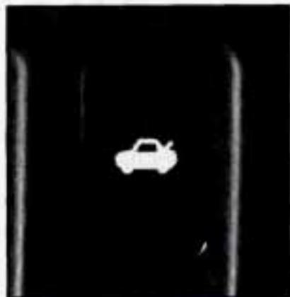
To use this feature, your vehicle must be in PARK (P) and the valet lockout button must be off. Press the trunk release button, located on the headlamp control panel on the left side of the instrument panel, to open the trunk.
