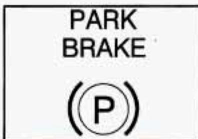
This light comes on when the parking brake is set, and it will stay on if the parking brake does not fully release. If you try to drive off with the parking brake set, this light will remain on.
