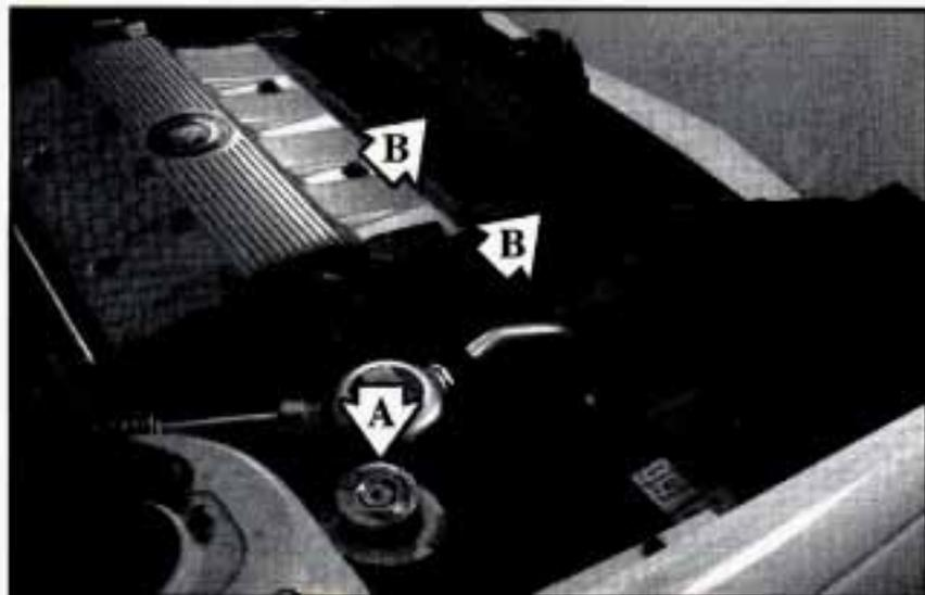
A. Coolant Surge Tank with Pressure Cap
