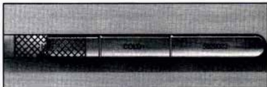
5. Check both sides of the dipstick, and read the lower level. The fluid level must be in the cross-hatched area.
