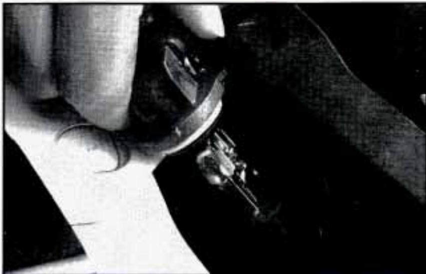
5. Reinstall the headlamp housing socket back into the headlamp assembly.
