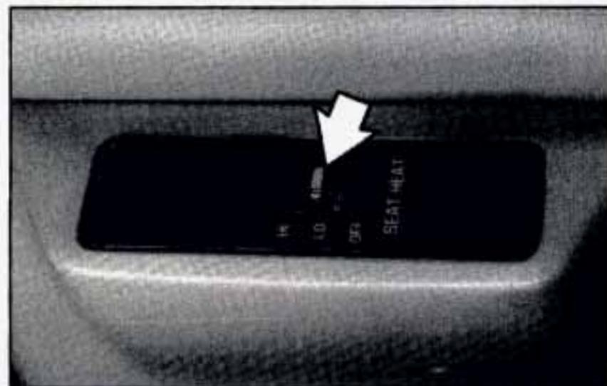
The control is located on the outboard side of each front seat. Move the SEAT HEAT control to either LO or HI
