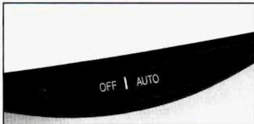
To turn on the automatic dimming feature, press **AUTO**. To turn off automatic dimming, press **OFF**. The green indicator light will be illuminated when this feature is active.
